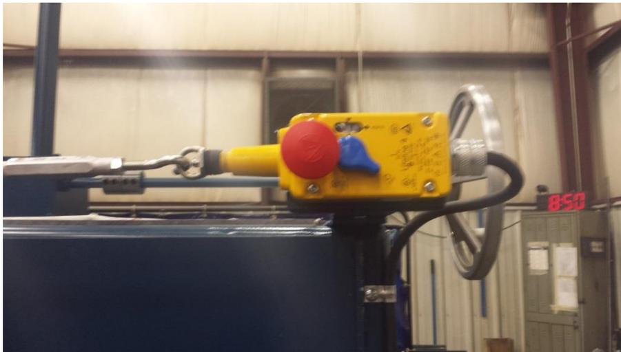
When the emergency cable has been tripped, the blue safety switch will be in the off position (lowered).
