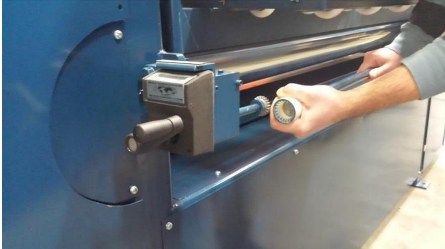
Depending on the set up of the machine, if you turn the coupling clockwise/or counterclockwise, it will move the doctor roll side that is furthest away from the unifeed handle either closer or farther away from the coating roll. Likewise, if you only turn the unifeed handle you can move the side closest to the handle either closer or farther away from the coating roll.
