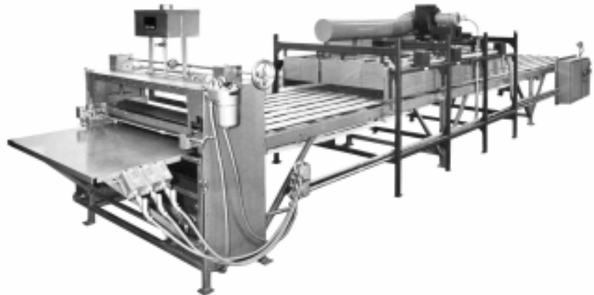
Roller coater applies liquid vinyl and heat sealing lacquer coating to cardboard stock. After coating, the material is moved via conveyor through a solvent flashoff area, then through an infrared oven that dries the applied film. A cool-out area permits stacking of material at the end of the line.
