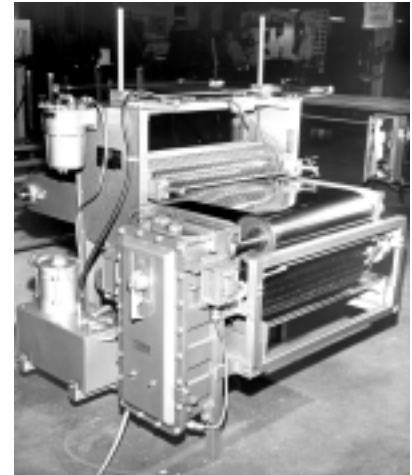
Gasket coater applies adhesive coating to thin gasket stock. Thru-conveyor is automatically cleaned with reverse-revolving brush roll.
