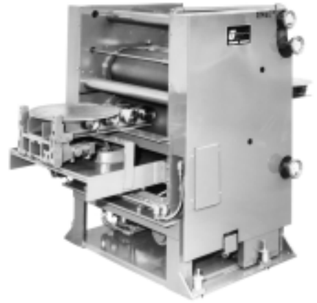
Drawing compound coater specifically designed to fit between columns of a transfer press. It will accept various sizes of stock parts.
