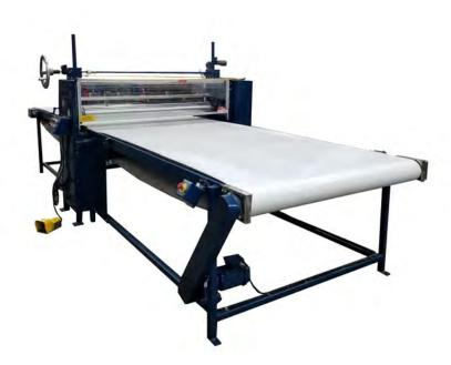
Our series 45 machine designed to roller coat waterbased adhesive to the top side of foam mattress pads.
