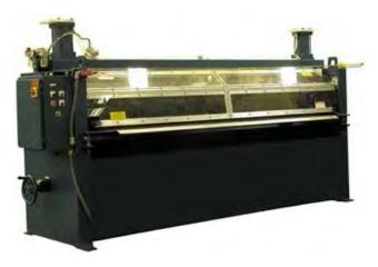
Our big Series #55, 120" Rotary Laminator is used to laminate RV sidewall panels after they are constructed.
