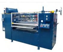
Our most popular roller coater used in the door industry is our Union Series #15, Model A- Hot Melt Roller Coater
