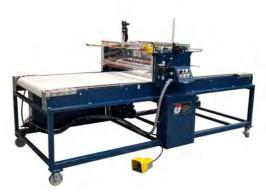
A smaller series 5 roller coater designed to apply a water-based adhesive to the top side of foam padded automotive parts.
