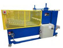
Drawing compound coater with return feed option eliminates offbearing labor. The return feed conveyor can be adapted to any Union Tool roller coater.
