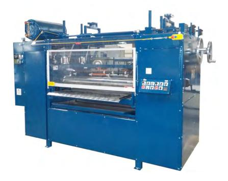
Union Tool's Hot Melt Roller Coater/ Hot Roll Laminator Combination Machine is an all-in-one type of machine. This machine combines the use of a hot melt roller coater, to apply hot melt adhesives, and a hot roll laminator, to laminate adhesive backed films, all under one framework machine.
