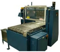
Drawing compound coater specifically designed to fit between columns of a transfer press. It will accept various sizes of stock parts.
