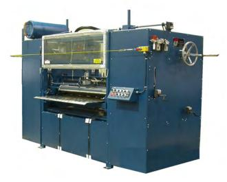
Union Tool's Dual Head Series #15, Model A/D, 54" Hot Melt Roller Coater. A double-sided hot melt roller coater that, with a flip of a switch, can be used as a single side coater without any downtime. This is one of our most popular machines used in the RV Industry today.
